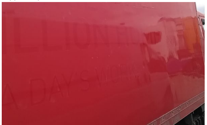
6: Wing nsf Poor Previous Repair Rippled Up To 30%
