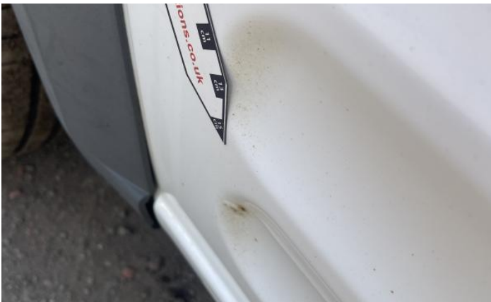
5: Door osf Dented With Paint Damage
