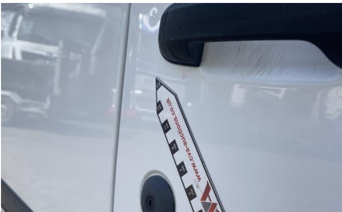
3: Wing nsf Dented Over 30mm
