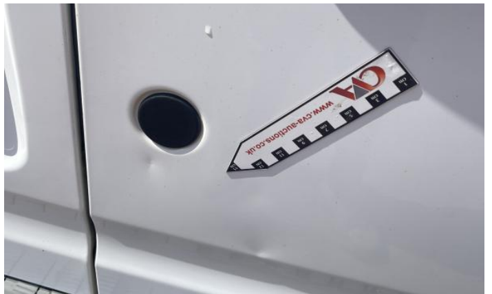
6: Sill os Rusted Over 5mm
